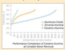
maintains its cut rate without needing significant additional pressure (see chart). This constant cut rate reduces grinding time, resulting in less operator fatigue, while increasing productivity and reducing abrasive costs.
