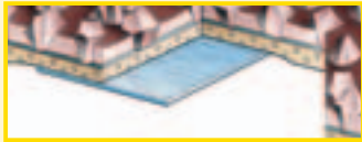
Type 4 butted joint with special film on the grit side
