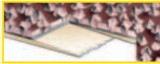
Type 2 overlapped joint with grit sanding
