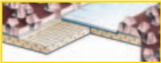
Type 3 butted joint with special film on the back
