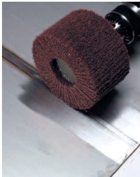
Example of a flap wheel made of Scotch-Brite™. Here the Scotch-Brite™ wheel is brushing the weld heat tint to blend the weld seam in with the surrounding metal. This finishing operation is not intended to flatten the seam. This would require an initial grinding operation.
