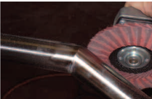
Treatment of the outside angle with flap disc abrasives
