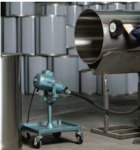
Flexible drive "flexi-polisher" machines usually use a heavy duty electric motor running on a 380 V power supply. This enables a wide range of powerful, but light finishing heads to be used. If very powerful, heavier units are used, this can limit the portability of the equipment.
